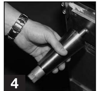
**4** Thread leg into cabinet bottom frame rail.
