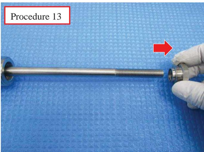
Remove Closing nut from Casing.
