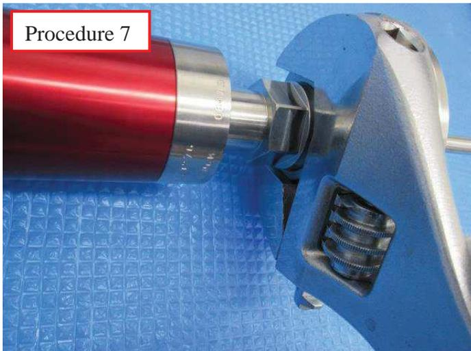
Hold the nut of Cover using open-end wrench or adjustable wrench.
