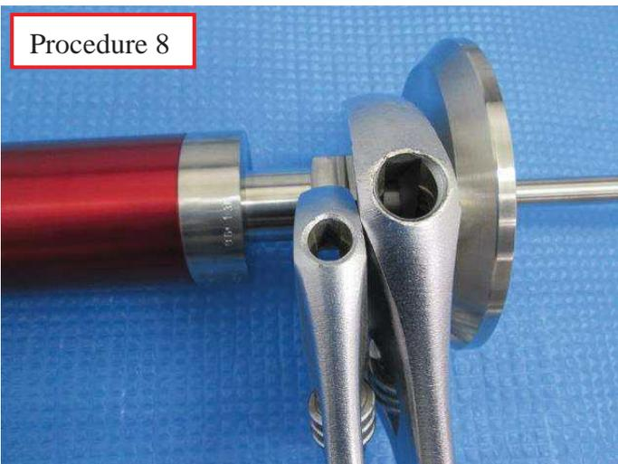
Hold the nut of Casing using open-end wrench or adjustable end wrench.
