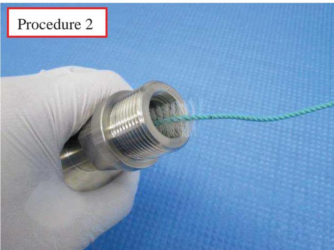
Polish using a soft brush to prevent any damage.
