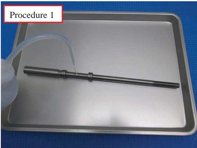
Pour the acetone to the Shaft using washing bottle.
