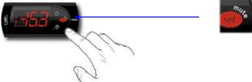
2. Press the up and down arrows to increase or decrease the set temperature. Then press the set button to save the new set point.
