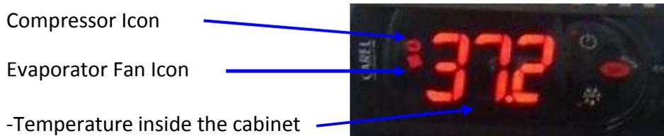
Verify you don't have any alarms on the temperature controller. If after you turn ON the equipment the controller shows the alarm icon or an error code, call for technical service. They will help you fix the problem.
